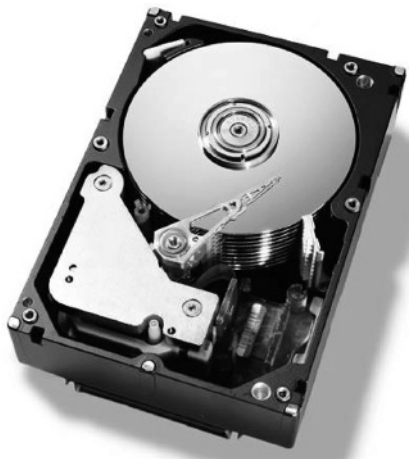
FIGURE 1.7 A side view of a multiplaten computer hard drive (from Ref. 34).
