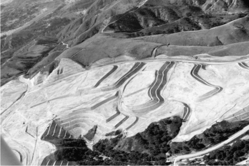
Figure 1.8 Alternative grading approach on a broad, round slope feature. Grading created terraced slopes and building pads but nevertheless replicated the underlying landform.
