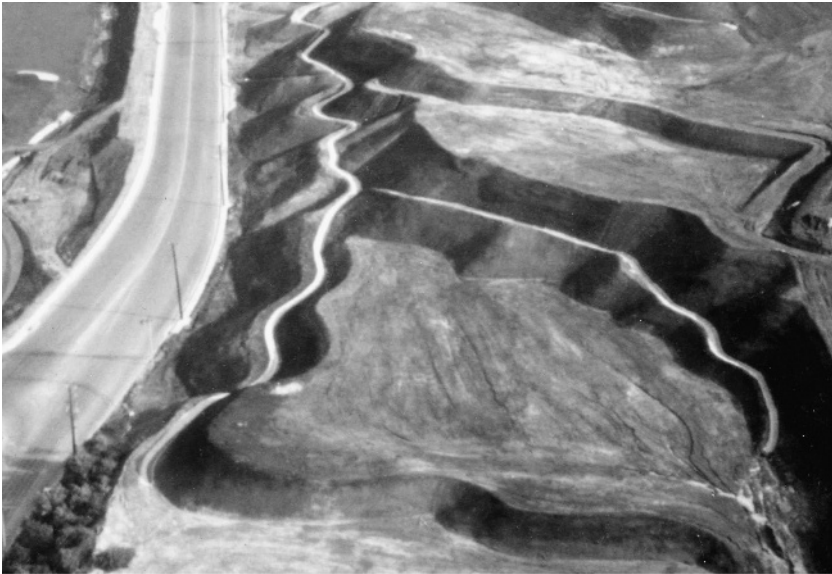
Figure 1.6 Photograph illustrating landform grading approach in a hillside development project in California.
