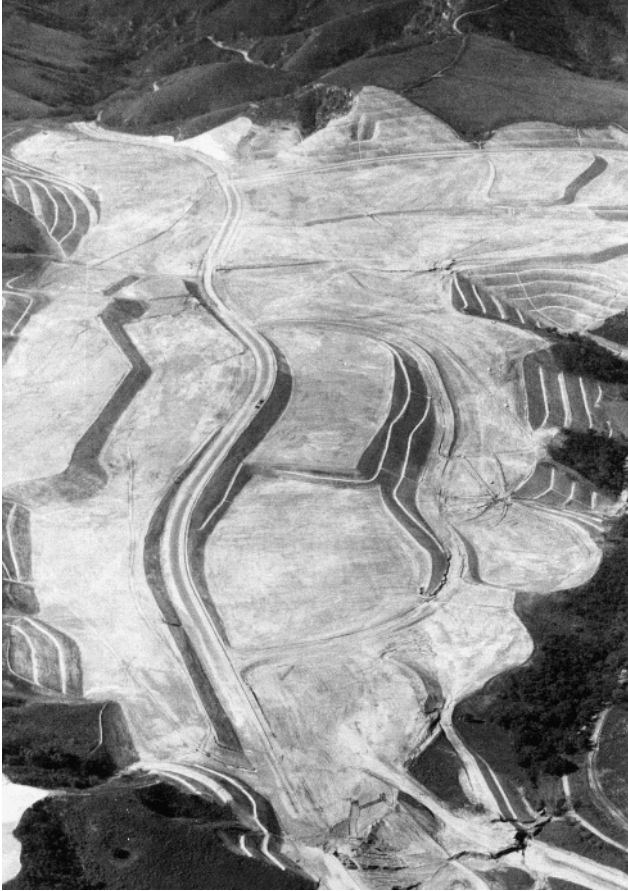
Figure 1.7 Conventional grading that cuts across secondary ridges and valleys, resulting in a terraced, stair-stepped landscape that obliterates the original terrain features.
