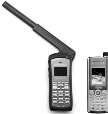
Figure 1.3 Handheld dual-mode satellite phones (Not to scale) used in: (a) a low-Earth-orbit satellite system. Courtesy © Globalstar; (b) a geostationary satellite system. Courtesy © Thuraya.
