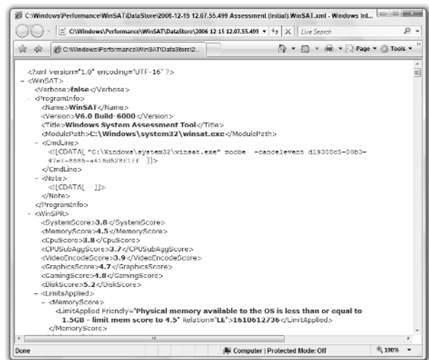
• Figure 1-8: The full, raw results that get massaged to produce your Windows Experience Index.
