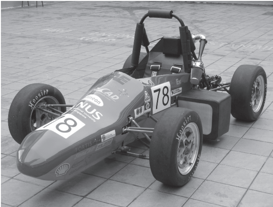
Figure 1.5. NUS-FSAE Car using Mg alloy in wheel assembly. (Courtesy: Professor K. H. Seah, National University of Singapore.)
