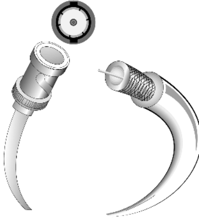
FIGURE 1.11 A male and female BNC connector
