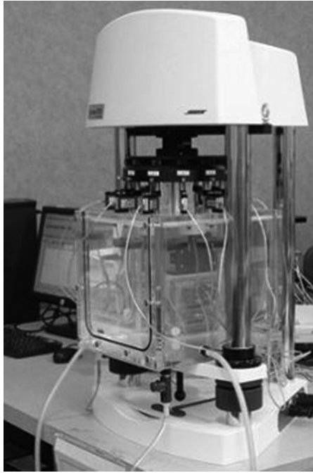
Figure 1.6. ElectroForce® multiple-specimen stent durability testing system [30].
