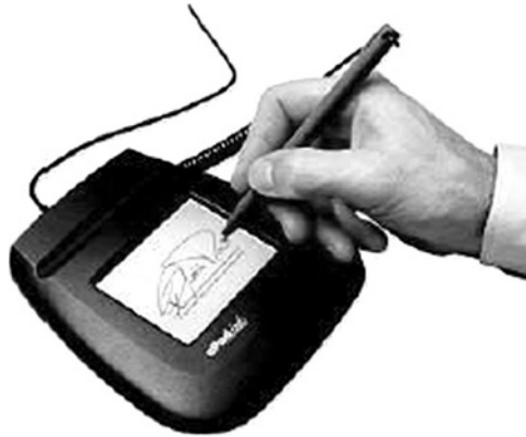
Figure 1.2 An online signature verification system (Source: Interlink Electronics ePad ( www.primidi.com/2003/05/31.html ))
