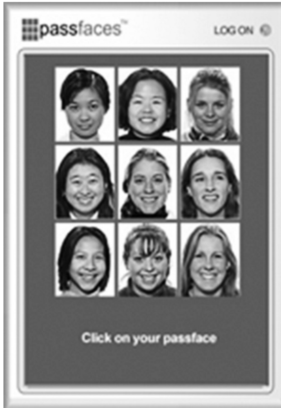
Figure 1.4 An example of the Passfaces™ graphical password authentication scheme. Note that on each page of faces, the user is required to select the correct face image; note that in this system, there is an implied order to the selection process (Source: Passfaces website – www.passfaces.com )
