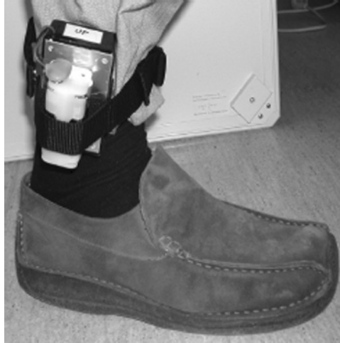
Figure 1.6 A photograph of a subject wearing a sensor-based gait device termed an accelerometer. Note that it is capable of measuring acceleration in three different orthogonal directions (Source: Gafurov et al., 2006)
