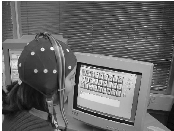
Figure 1.9 A subject interacting with a virtual keyboard while wearing a standard 10–20 electroencephalogram skullcap (Source: Internet image – www.lce.hut.fi/research/css/bci *Copyright requested)
