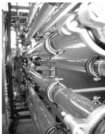
30 L pilot reactor for moss
