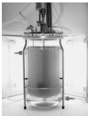
Fig. 8 Greenovation use a fully contained moss bioreactor. This company has established an innovative production system for human proteins. The system produces pharmacologically active proteins in a bioreactor, utilizing a moss ( Physcomitrella patens ) cell culture system with unique properties. Source: Knäblein J. (2003) Biotech: A New Era in the New Millennium – Biopharmaceutical drugs Manufactured in Novel Expression Systems , DECHEMA-Jahrestagung der Biotechnologen, Munich, Germany, 21.
