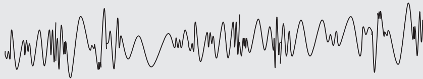
Figure 1.5 A representation of a groove on a vinyl record
