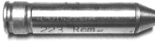
Figure 1.21 Rimless cartridge headspace gauge.
