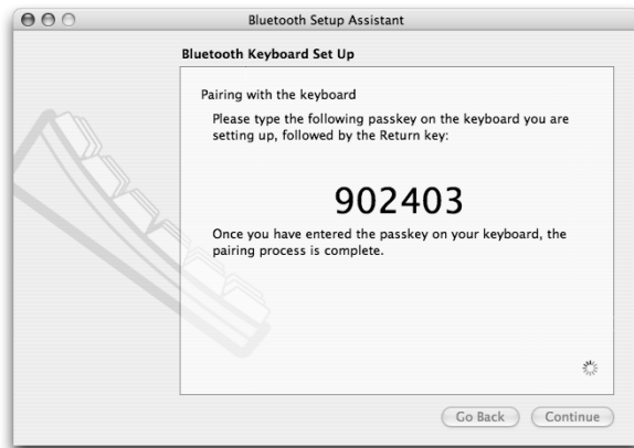
Figure BC1: You need to enter a passkey to pair two Bluetooth devices.
