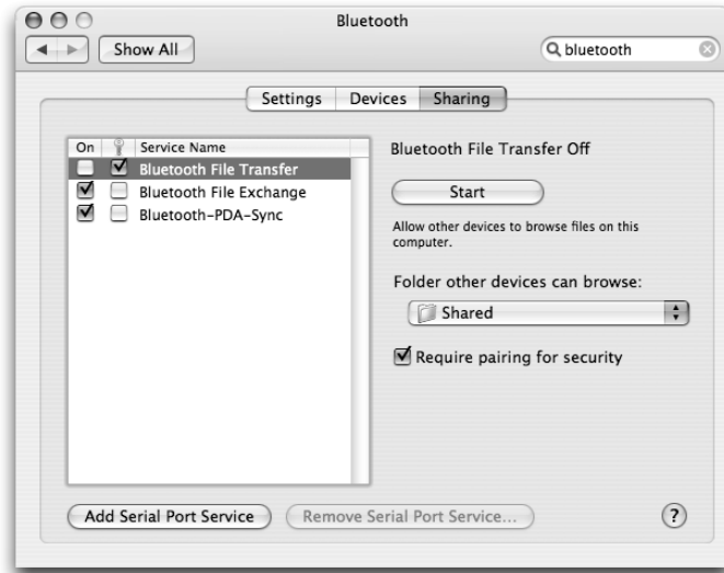
Figure BC10: You can control the specifics of Bluetooth file sharing from this preference tab.
