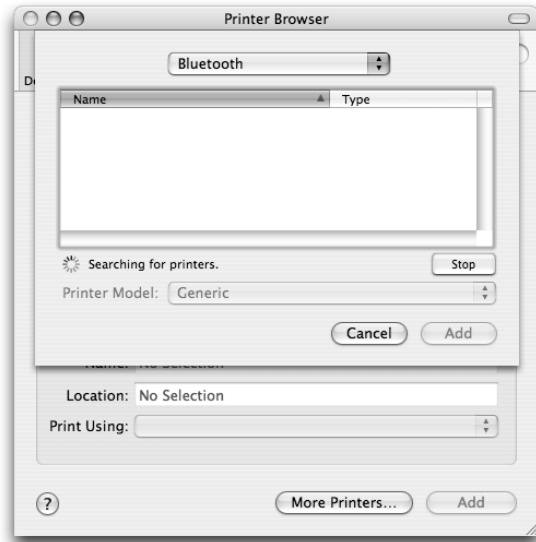
Figure BC43: Choose Bluetooth from the pop-up menu to find nearby Bluetooth printers.
